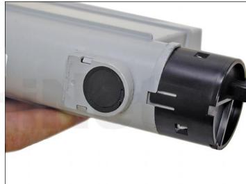
8. Snap the chip holder back on the cartridge.
